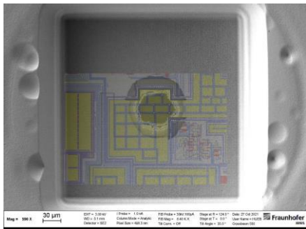
Fig. 2: P-FIB backside trenching of the Si substrate overlaid with the IC layout of the ROI, before and after detailed Ga-FIB investigation
