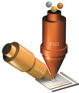
Left: General VELION setup with vertical FIB column, Laser Interferometer Stage and SEM
